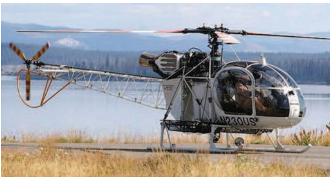
FIGURE 116-7 Wildland fire helicopter H 1109, a rental helicopter from Inyo National Forest (Aérospatiale SA 315B Lama, not litter capable) used in Sequoia and Kings Canyon National Park. These helicopters are not designed for medical rescues and do not accommodate supine patients, even in emergencies. (Courtesy Jason Bauwens.)
