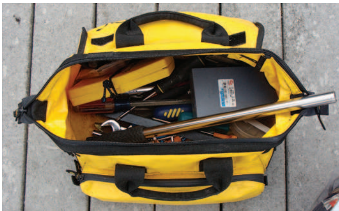
FIGURE 70-13 Damage control kits are not suitable for making fine furniture; in fact, one may have to remove the furniture in the vessel's saloon to get to the source of the leak. Saws, hammers, rivet tools, Band-It tools, and a rechargeable drill are just some of the items one needs to carry.
