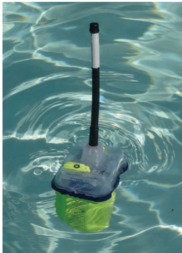
FIGURE 70-27 EPIRBs float upright and can transmit while bobbing in the water next to a life raft or damaged vessel. They include a tether that must be attached to the vessel or raft so that the EPIRB does not drift away.
