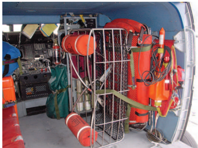
FIGURE 70-34 The interior of an MH-60 Jayhawk is crowded, even before the survivors are taken onboard. The basket, rafts, and pumps can be seen in the photo. This gear can be jettisoned if room is needed for rescued mariners.
