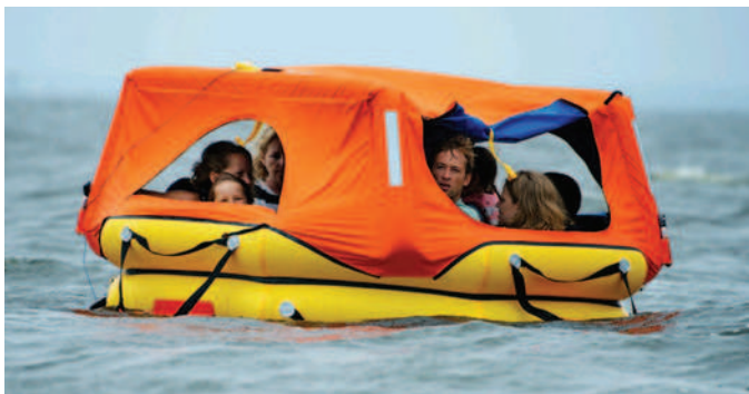
FIGURE 70-29 Example of a modern offshore life raft. There are lots of options for adjusting visibility and ventilation, excellent ballasting, and redundant buoyancy.
