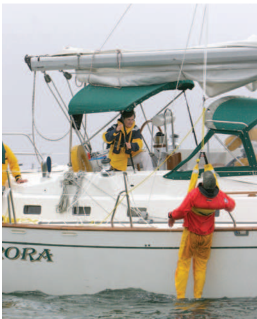
FIGURE 70-10 Getting the person in the water back onboard is not a simple task. The Lifesling provides flotation, connects the victim to the vessel, and serves as a lifting sling.
