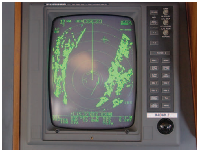
FIGURE 70-19 Although radar reflectors make a vessel incrementally more visible on a ship's radar, it is a lot easier for you to see them than vice versa. Keeping a radar watch in shipping channels makes sense, as it does here in the Strait of Juan de Fuca.
