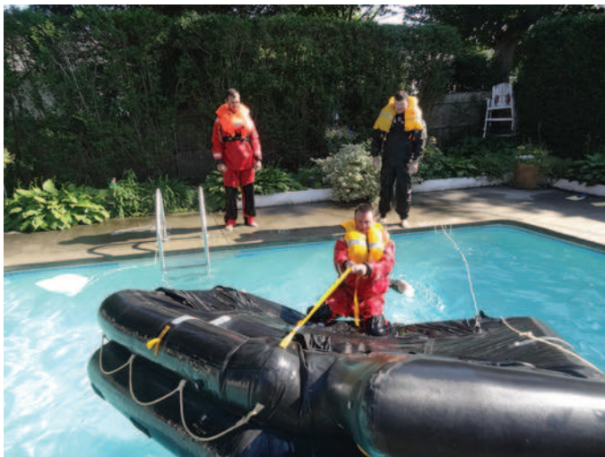
FIGURE 70-32 Righting a life raft is not difficult, but remember to keep the inflation bottle (cylinder) close to the feet so that it does not strike one on the head.
