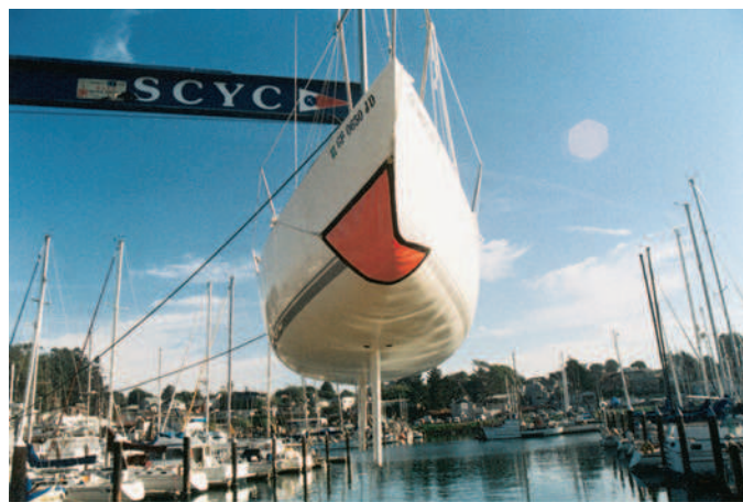
FIGURE 70-16 A collision mat consists of a triangular piece of fabric that is held in place with lines attached to each corner. Water pressure and the lines hold it in place.
