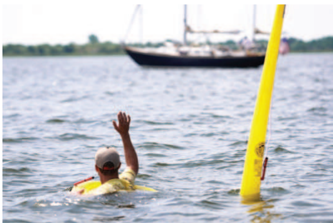
FIGURE 70-6 This crew overboard module consists of an inflatable horseshoe-shaped buoyant device, 1.8-m (6-foot) inflatable locator pylon with a light, and self-opening sea anchor.
