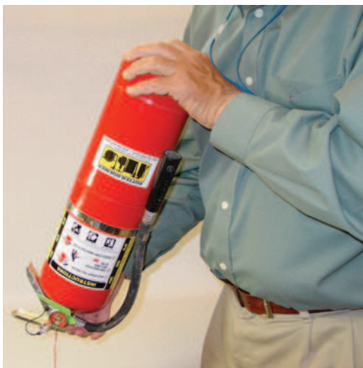
FIGURE 70-12 Dry chemical fire extinguishers should be inspected to ensure the pressure gauge indicates a full charge, and should be inverted regularly to unpack the extinguishing agent.
