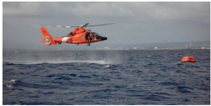
FIGURE 70-33 Coast Guard MH-65 helicopter off of Pearl Harbor, Hawaii. With a duration of about 3 hours, the MH-65 is used within 100 miles of the coast.
