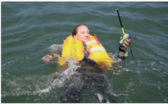
FIGURE 70-9 A personal locator beacon (PLB) may be an excellent link back to the Coast Guard, but if you are too far offshore, you may not survive until the Coast Guard arrives. Consider a MOB beacon that alerts the crew on the mother ship, or better yet, both methods.
