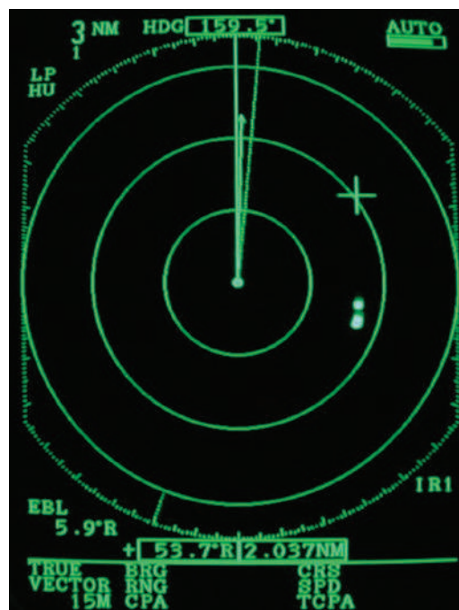
FIGURE 70-20 Plotting aids, such as ARPA and MARPA, remove much of the doubt about whether or not the other vessel is going to pass safely.
