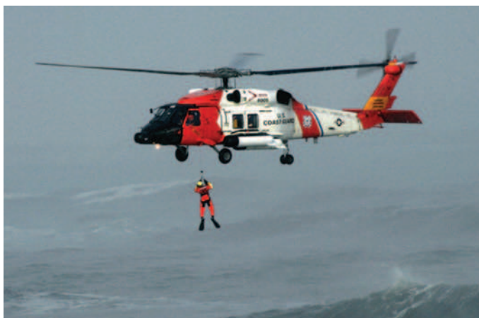
FIGURE 70-35 Rescue swimmer being hoisted by an MH-60 Jayhawk with a lifting sling.
