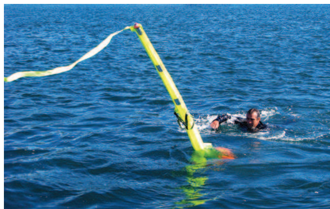
FIGURE 70-7 The MOB Dan Buoy is a ballasted, inflatable pylon with a light at the top, very visible streamer, drogue, and enough buoyancy to float the victim.
