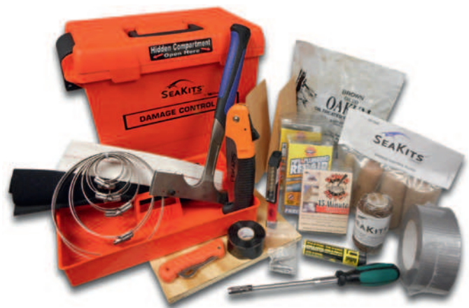
FIGURE 70-15 A damage control kit focused on flooding. Tapered wooden (or foam) plugs, underwater epoxy, saws, and hose clamps provide a variety of tools to stem the flow. (Courtesy WheelHouse Technologies, Inc, Hudson, MA.)
