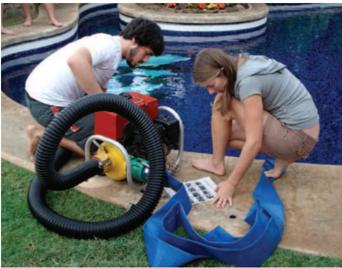
FIGURE 70-17 Coast Guard gasoline-powered dewatering pumps are extremely effective, but are also a bit cryptic in their use. Note that she is reading the waterproof instructions, while he ponders the controls. Some are self-priming, while others may have a hand pump to draw water into the pump body.
