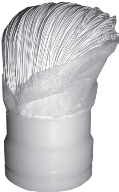
FIGURE 88-30 Microtubules in Sawyer filter cartridge. (Courtesy Sawyer Products.)
