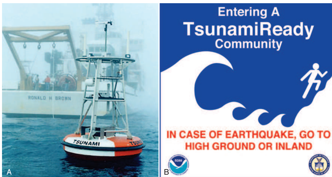
FIGURE 17-29 A, Tsunami buoy contains pressure sensors for determining a wave's size by gauging the weight of the water column passing over it. B, "TsunamiReady" sign. (Courtesy National Oceanic and Atmospheric Administration.)
