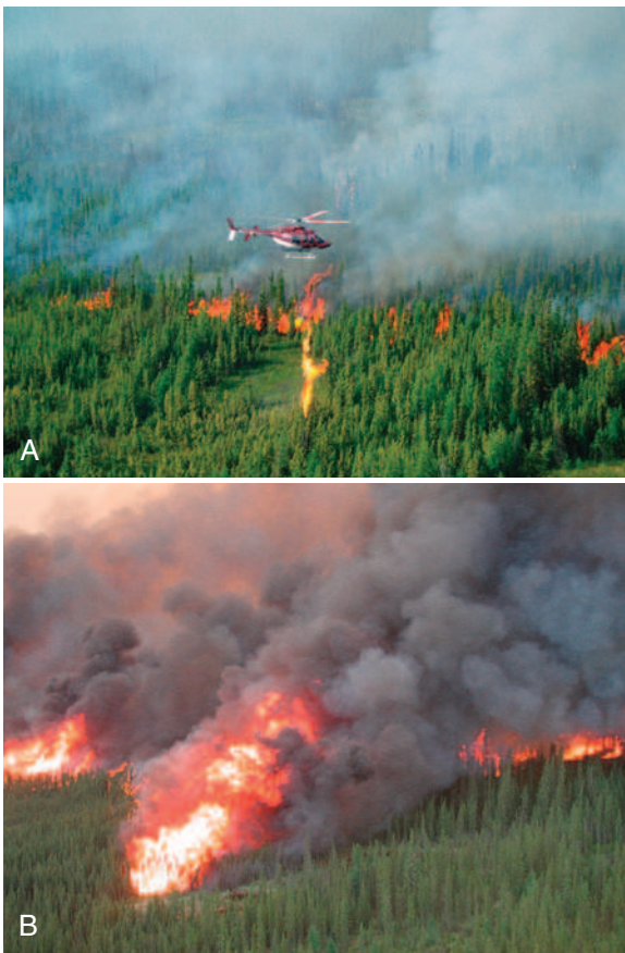
FIGURE 14-3 A helitorch, or flying drip torch, is a specialized aerial ignition device slung below and activated from a helicopter (A). It dispenses and ignites gelled fuel. The use of a helitorch in wildfire suppression operations can take many forms (e.g., to reduce fire intensity; to slow or steer a fire; to remove potentially dangerous fuel concentrations; to widen and strengthen control lines; to expedite mop-up operations). Regardless of its specific purpose, the main objective of this application of “fighting fire with fire” is to speed up or strengthen control actions (B). Aerial backfiring and burning out with a helitorch can be one of the safest, most economic, fastest, and least damaging means of widening control lines and constitutes one of the major innovations in wildland fire suppression technology in the past 35 years. The helitorch is also used in prescribed burning operations. (Courtesy Alberta Sustainable Resource Development and Wildfire Consulting Ltd, Edmonton, Alberta; photos by O. Spencer and W. Bereska.)
