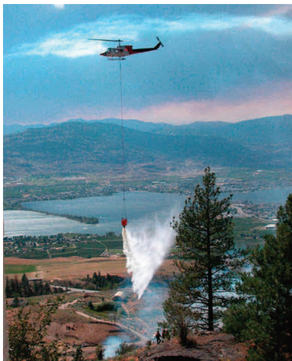
FIGURE 14-5 Several different sizes and models of rotary-wing aircraft or helicopters are used in a wide variety of direct roles as well as support functions in wildland fire suppression, including the dropping of water or fire-retarding chemicals directly on the fire. Helicopters also create wake vortices while in forward motion, just like airplanes, but generally these vortices are much weaker. A more common safety issue with helicopters is the downward induced air flow or rotary downwash. Some downwash effects are unavoidable when helicopters are engaged in direct attack on the fire with water or chemicals. Anyone located near the fire perimeter during such operations could be at risk. Even with a “long line” delivery system operated from a Bell 212 helicopter, as illustrated here on the Anarchist Mountain Fire near Osoyoos in southern British Columbia on July 16, 2003, rotary downwash can still be a significant issue. (Courtesy Alberta Sustainable Resource Development.)
