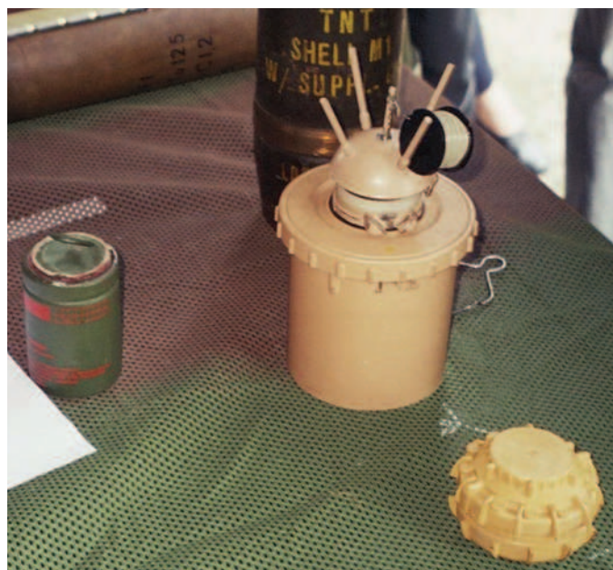
FIGURE 86-4 Land mines. From left to right, M14, Valmara 69, and VS-50. (From Nation Defense Days, Esplanade des Invalides, Paris, France, September 24 and 25, 2005. )
