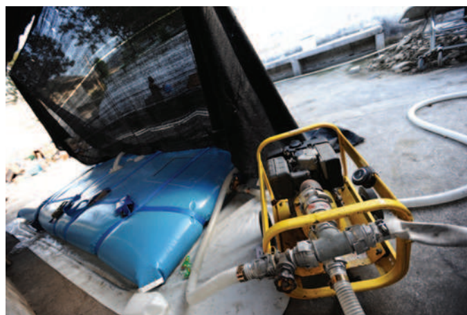
FIGURE 84-44 Water pump and water bladder equipment used for kidney dialysis at Port-au-Prince General Hospital following the 2010 earthquake in Haiti. (Courtesy Julie Remy, Médecins Sans Frontières.)
