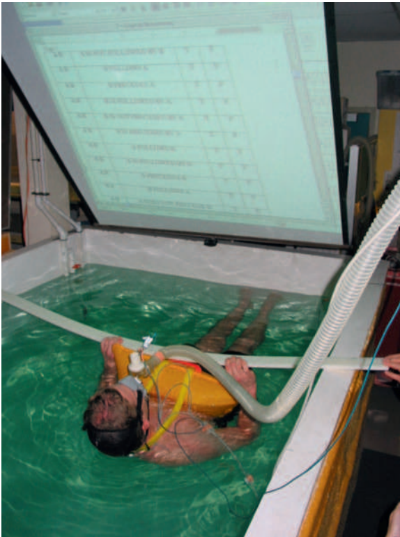
FIGURE 8-25 Cognitive function testing in a participant wearing a prototype inflatable personal flotation device in a study to assess the relative contributions of the dorsal head and the body to core-temperature decline and cognitive function in cold-water immersion.
