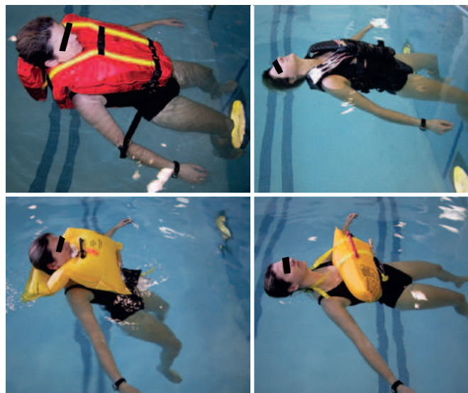
FIGURE 8-21 Effectiveness of various types of personal flotation devices for keeping the head and the upper chest out of the water. Top left, Type I jacket; top right, type 3 jacket; bottom left, typical keyhole inflatable jacket; bottom right, waist-mounted inflatable device. (Courtesy Gordon G. Giesbrecht.)
