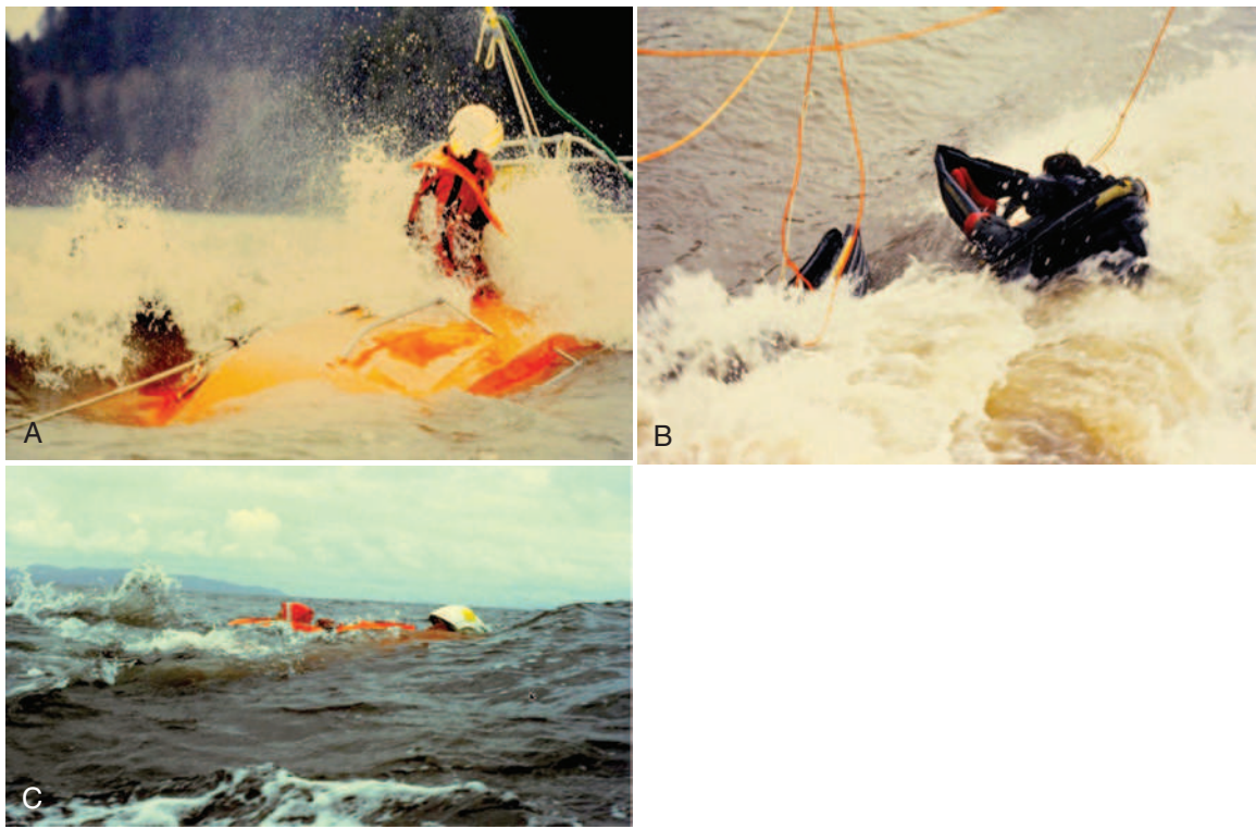
FIGURE 8-36 Testing protective clothing in rough seas: A , atop an overturned boat; B , in a one-person life raft; C , free swimming with only a personal flotation device. (Courtesy Alan Steinman)
