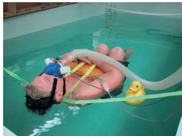
FIGURE 8-27 Participant adopting the heat escape lessening position (HELP) while wearing a prototype inflatable personal flotation device in a study to assess the relative contributions of the dorsal head and the body to core-temperature decline and cognitive function in cold-water immersion.
