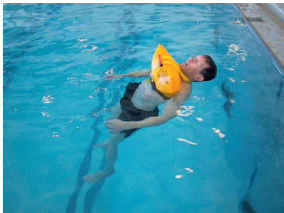
FIGURE 8-28 Investigator testing the flotation posture of a prototype inflatable personal flotation device in an “unconscious” survivor.
