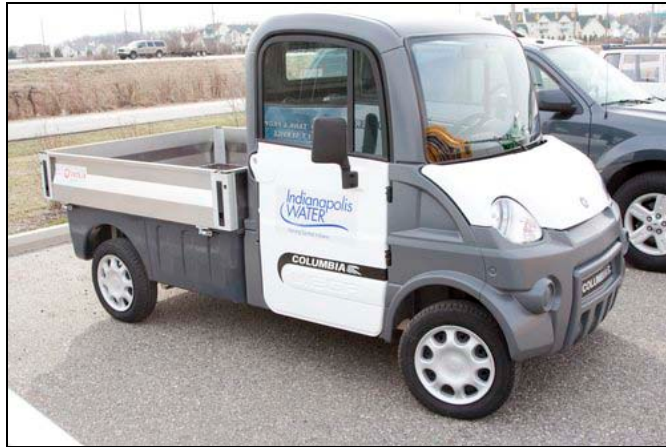
Figure 2-2: NEV - Neighborhood Electric Vehicle for Utility Purposes (Photo courtesy of NREL Photographic Information Exchange)
