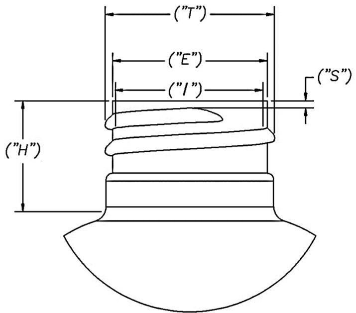
"I" Dimension: The inner diameter of the bottle neck. Specifications require a minimum "I" to allow sufficient clearance for filling tubes. Linerless closures, with a plug or land seal, and dispensing plugs and fitments require a controlled "I" dimension for a proper fit.
