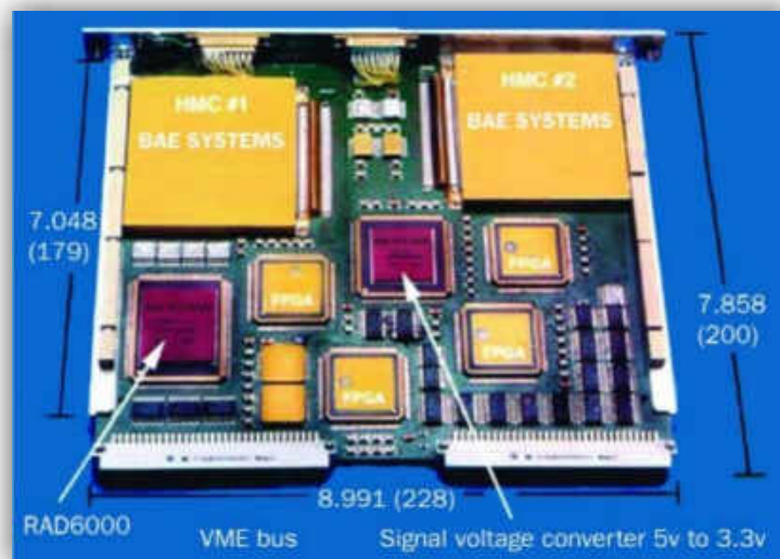
Mars Rover Flight Computer. © Lockheed Martin, BAE
