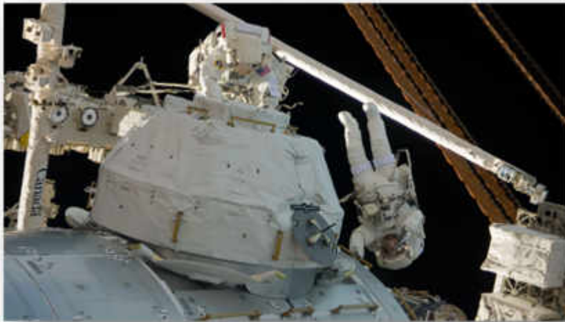
During the mission's third spacewalk, Nicholas Patrick, Left, and Robert Behnken remove thermal blankets from the cupola.
