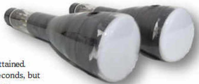
RCA 6571 Williams Tubes, used in early computers such as the IBM 701, also in my collection.
