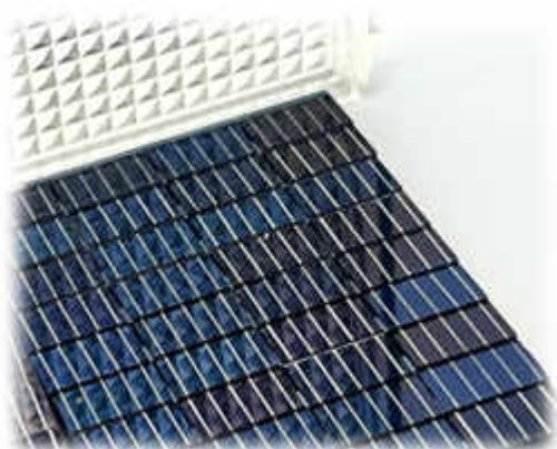
The display opened, showing the solar cells themselves.
