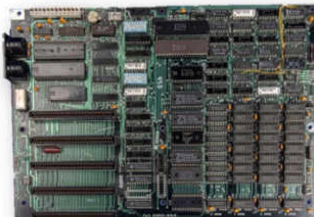
No fans or heatsinks, the Intel 8088 is just another chip on this board. German / CC BY-SA 3.0
