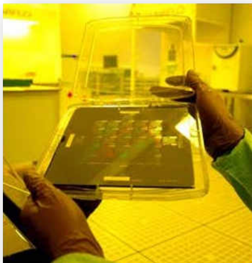
Chromium mask used for photolithography.
