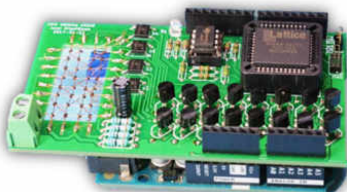
An Arduino with a tiny DIY core memory plane setup. © David Ives
