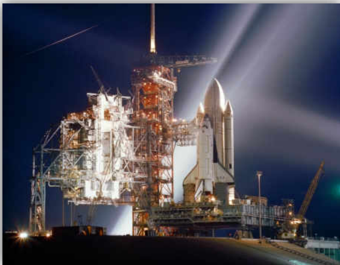
Looking majestic on the launchpad. Note the white external tank, this paint job was omitted on later flights to save weight
