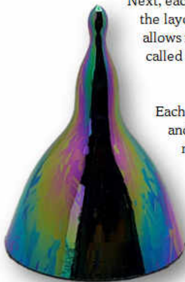
Rainbow-hued end piece of a silicon boule; also in my collection.
