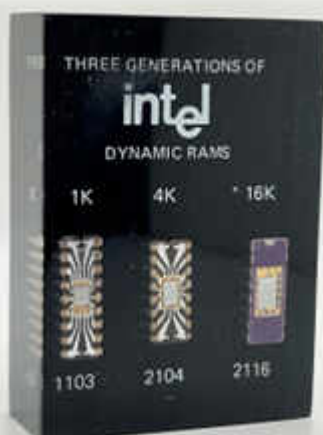
Lucite with 1103 and successive generations of Intel DRAM, also in my collection.
