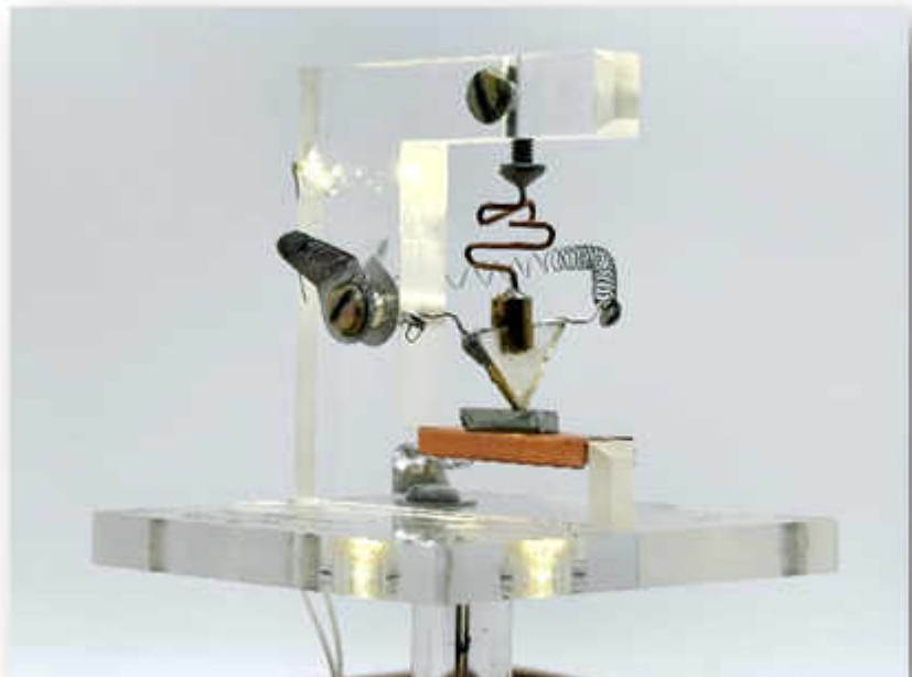
A replica of the first transistor, also in my collection.
