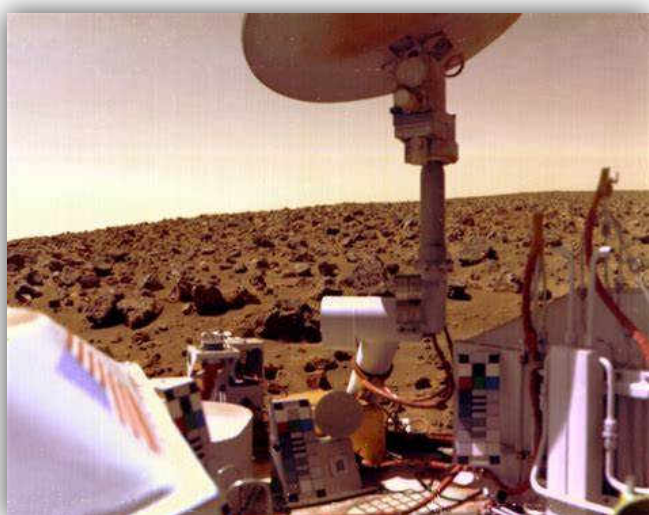
First Mars selfie, note the camera calibration marks at the base of the antenna mast.
