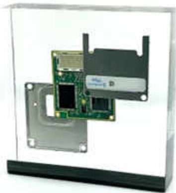
The reverse, note the connector on the chip which allowed for a very flush mount.
