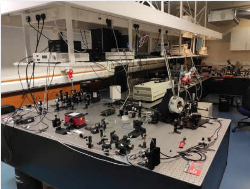
The Quantum Photonics Lab at the University of Southampton, furnished with three ultralow-vibration optical tables surmounted by an overhanging rack for electrical equipment. The tables are equipped with various lasers, and a confocal microscope is devoted to the study of color centers and their coupling to optical devices. Three waveguide characterization setups can be used for non-linear and quantum measurements (including single photon counting).
