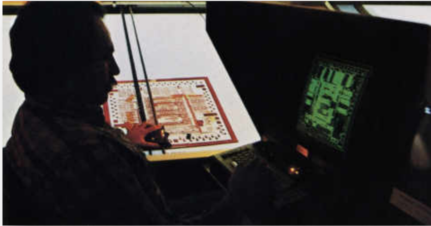
This circuit diagram will be reduced hundreds of times before it is used.
