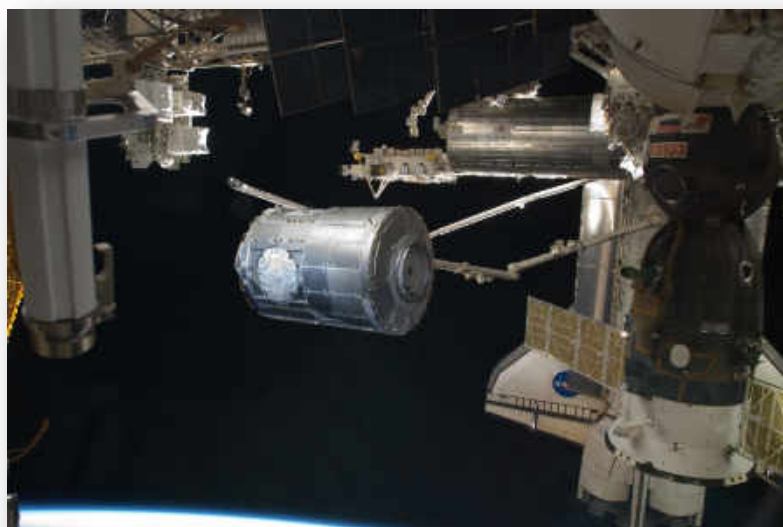
In the grasp of the station's Canadarm2, the Tranquility module is transferred from its stowage position in space shuttle Endeavour's payload bay to position it on the port side of the Unity node of the International Space Station. Tranquility was locked in place with 16 remotely-controlled bolts.
