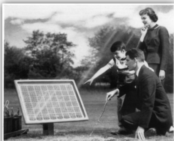
Something New Under the Sun. It's the Bell Solar Battery, made of thin discs of specially treated silicon, an ingredient of common sand. It converts the sun's rays directly into usable amounts of electricity. Simple and trouble-free. (The storage batteries beside the solar battery store up its electricity for night use.)
