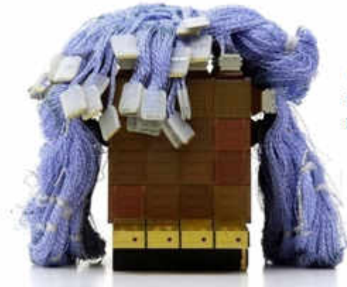
The Cray-3 used a three-dimensional module design, with a constraint of one-foot maximum wire length to enhance performance and reduce size. © Mark Richards. Courtesy of the Computer History
