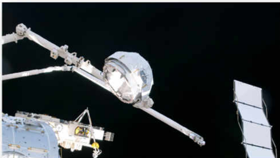
Relocation of the cupola to Tranquility's Earth-facing port.
