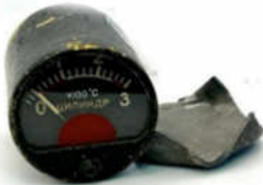
This Soviet temperature gauge uses ra-226 to glow in the dark and helpfully came with a piece of lead.
