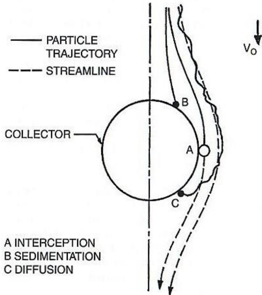
**FIGURE 10-10** Basic transport mechanisms in water filtration.
