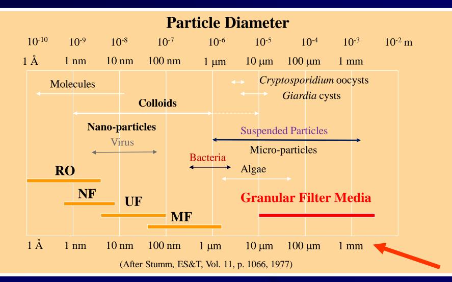
Relative size of particles in settled water as compared to of 1 mm anthracite grains mm
