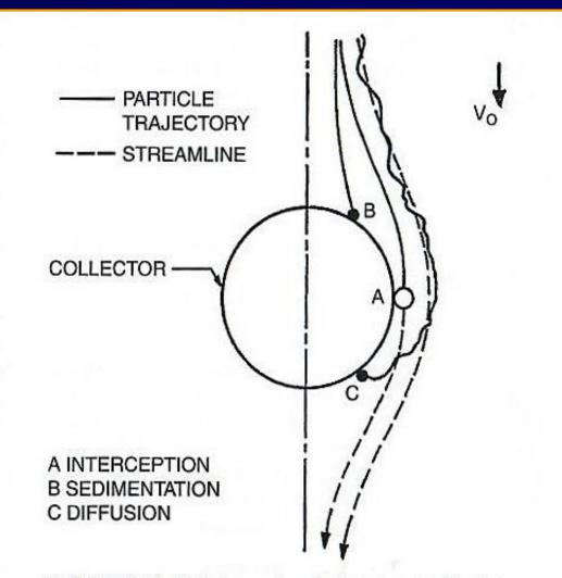
FIGURE 10-10 Basic transport mechanisms in water filtration. (Source: Reprinted with permission from Yao et al., 1971.)
