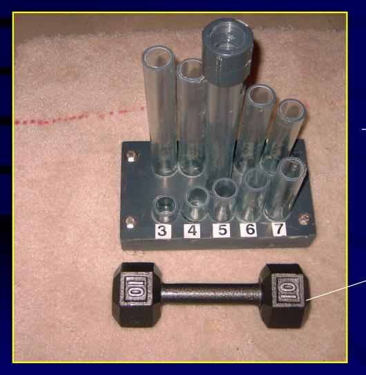
Make the expansion tool out of good heavy materials so it holds up under repeated use
