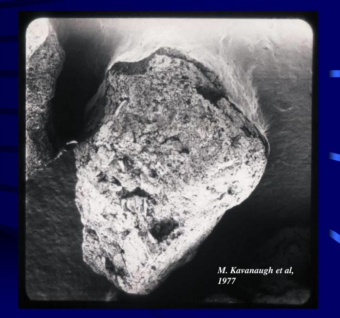
Scanning Electron Micrograph Anthracite Filter Media, 1 mm
