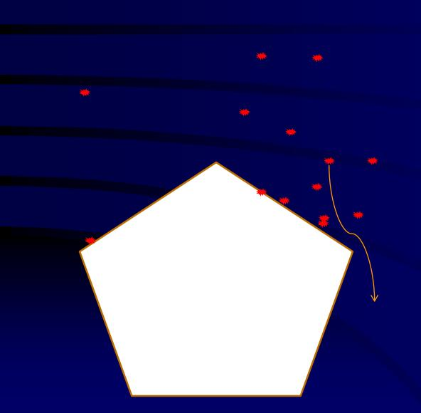
Filtration is "transport and attachment" of floc particles in the water
