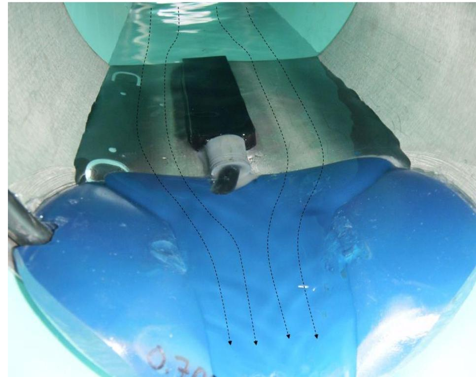
Low Profile Probe Flow Low Flow Applications
