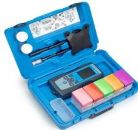
Easy Field Testing w/ up to 6 parameters at once.
