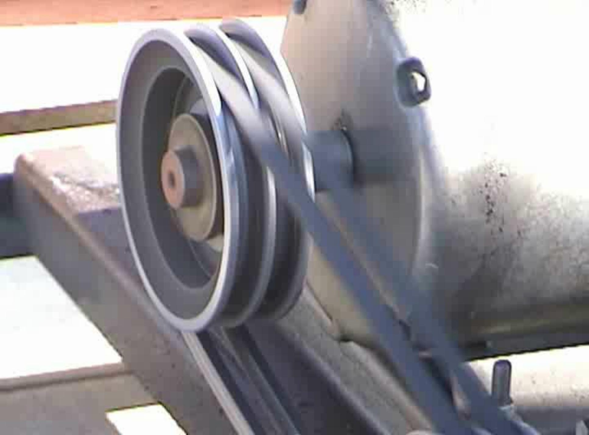
A V belt transfers power by friction and the mechanical advantage of the wedge-shaped section of the sidewalls, not the bottom.
