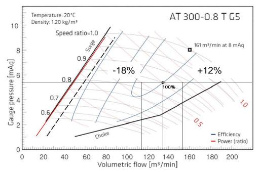
Controlling the flow through current instead of speed achieves greater flow precision
