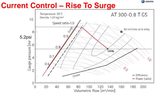
Controlling the flow through current instead of speed achieves greater tolerance to pressure spikes
