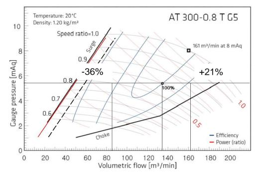
A variation of  $\pm$  5% in speed is equivalent to a variation of + 21% and -36% in flow
