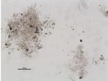
Figure 13-SBR 1 Foam unstained and viewed with 100X magnification showing clumps of branched filaments and trapped fine particles including septic particles.
