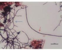
Figure 15-SBR 1 Foam Gram stained and viewed with 1000X magnification showing Nocardioforms (blue arrow) and *M. parvicella* (red arrow).
