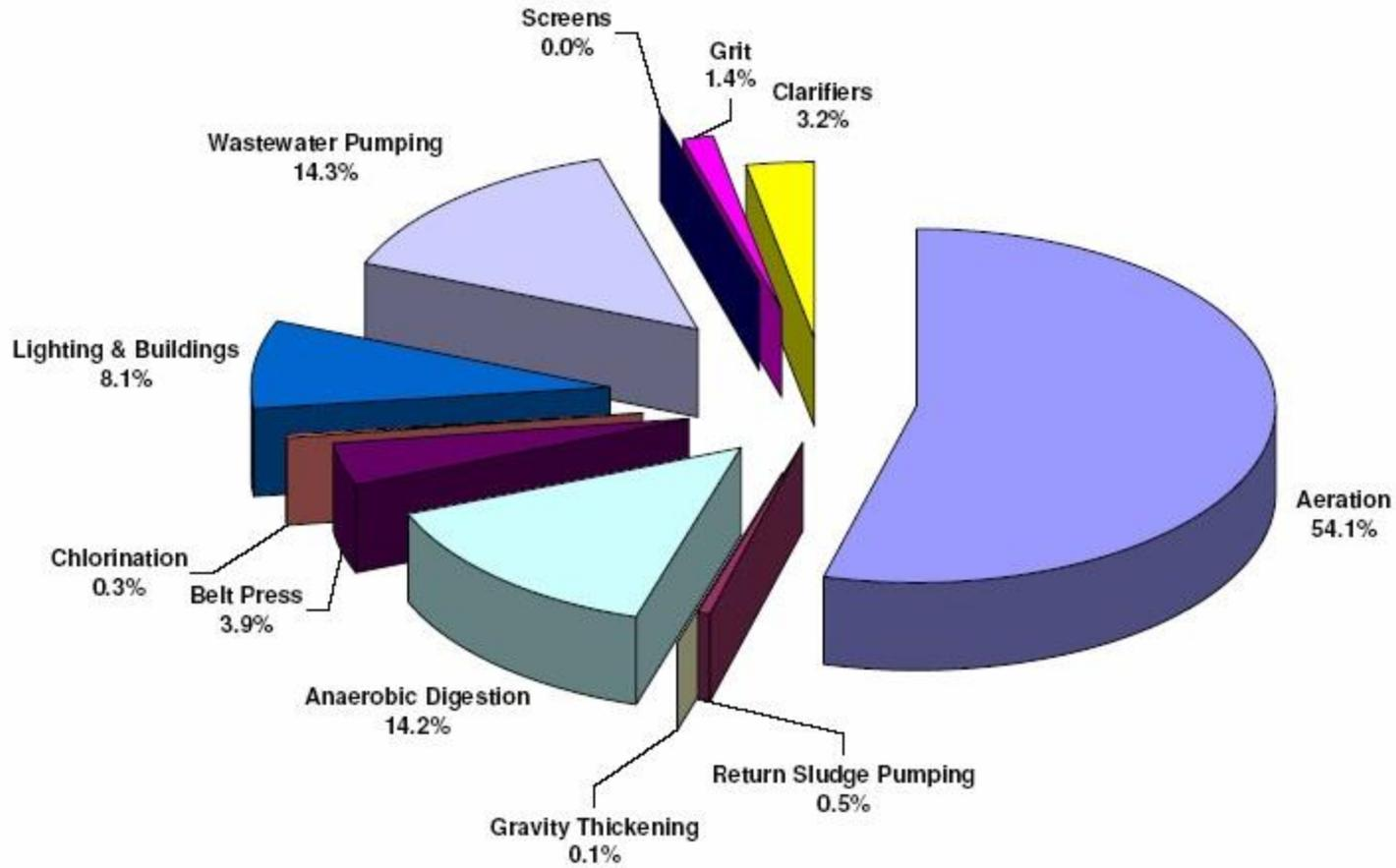
Typical Power Consumption in Activated Sludge Processes
