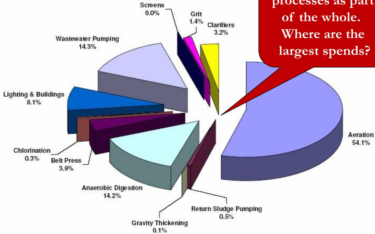
Typical Power Consumption in Activated Sludge Processes
