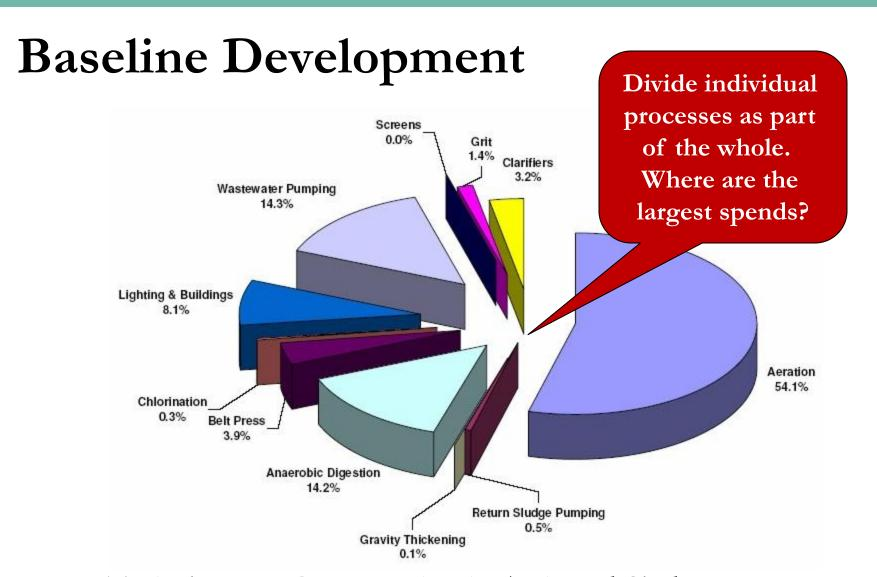
Typical Power Consumption in Activated Sludge Processes
