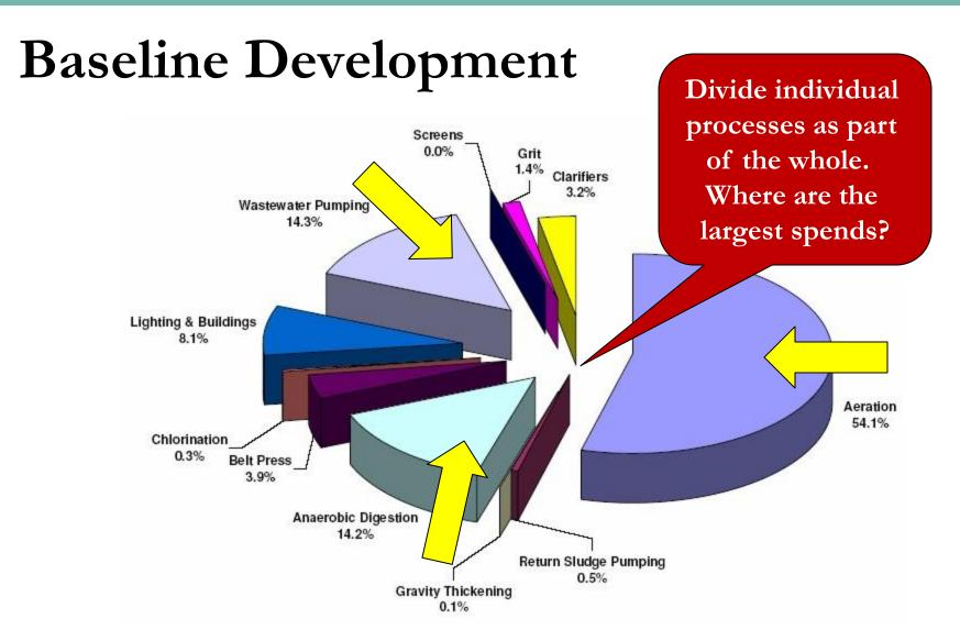
Example Power Consumption - Activated Sludge Processes
