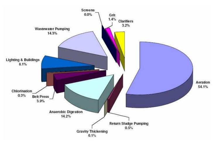
Typical Power Consumption in Activated Sludge Processes
