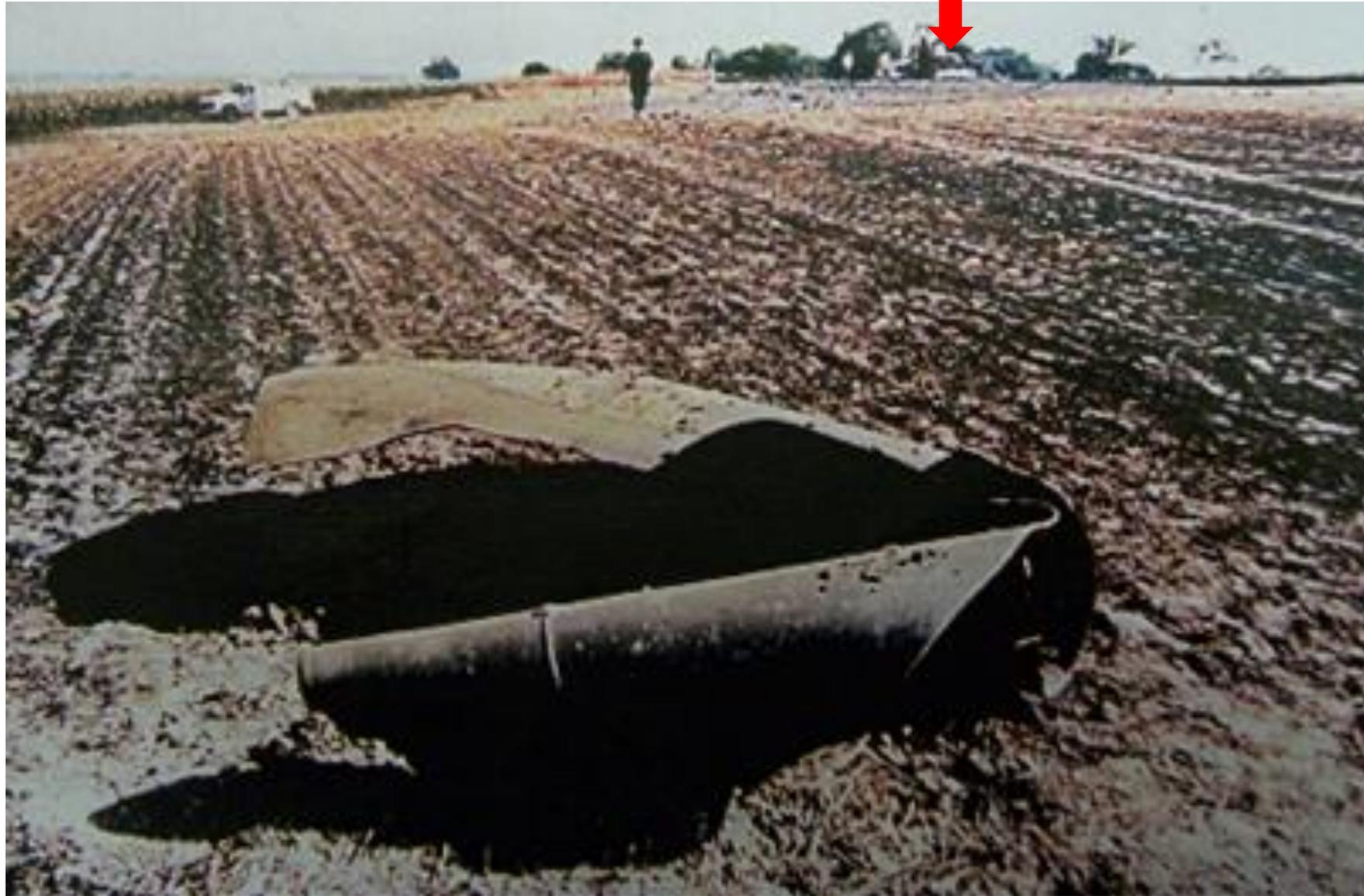
This image shows a piece of the pipe section thrown from the accident site
