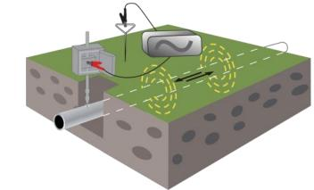
• Active Locating – Signal produced by transmitter and located using the receiver
