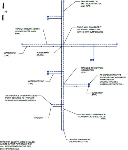
WIRE SHOWN AWAY FROM PIPE FOR CLARITY, WIRE SHALL BE INSTALLED ON THE BOTTOM SIDE OF THE PIPE BELOW THE SPRING LINE. THE WIRE SHALL BE FASTENED TO THE PIPE WITH TAPE OR PLASTIC TIES AT 5' INTERVALS.
