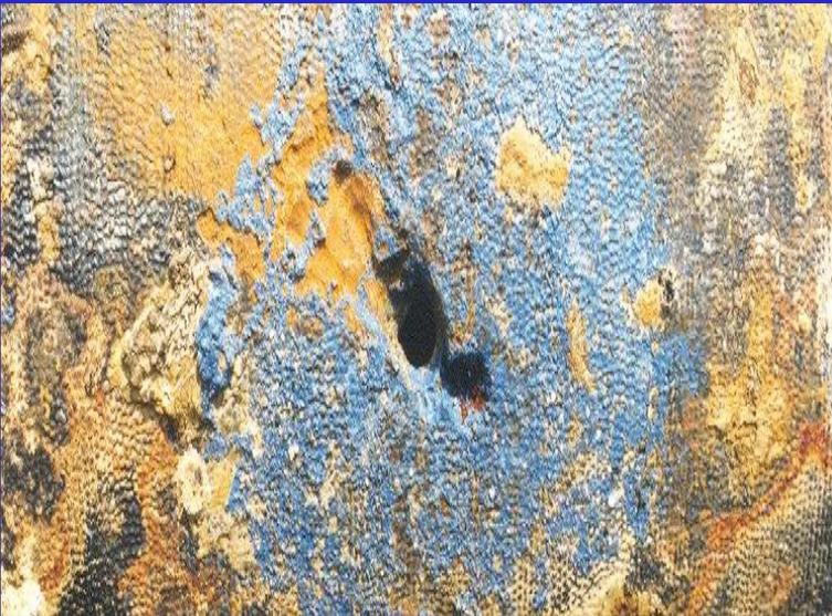
Pitting (concentrated) corrosion attack on ductile iron pipe.
