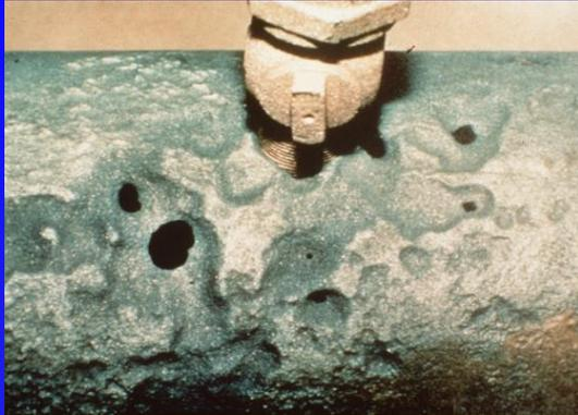
Corrosion of iron when coupled to copper service line.
