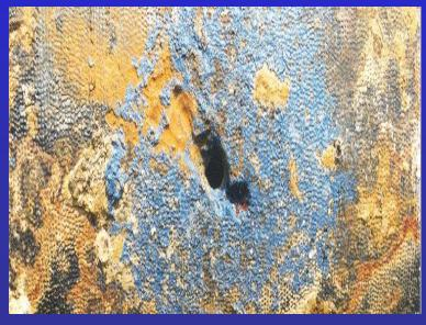
Pitting (concentrated) corrosion attack on ductile iron pipe.
