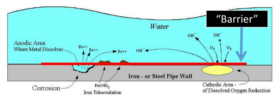
A "Coating" is laid down to shut down the process. Some phosphates are better at Anodic Corrosion and others better at Cathodic
