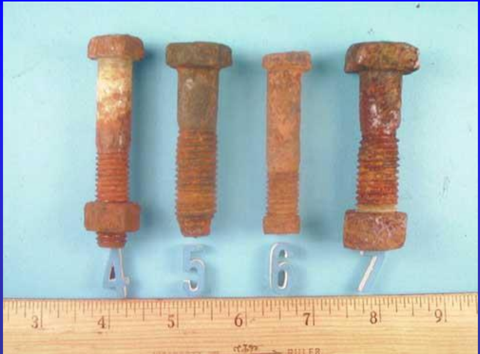
Bolt & Nut Corrosion
