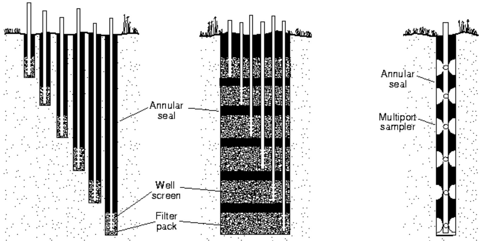
(a) Monitoring wells with short screens, each installed in its own borehole
