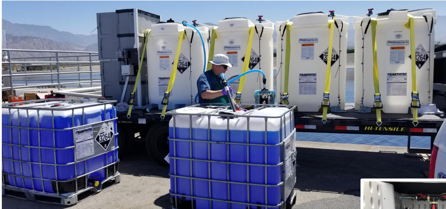
EarthTec liquid ionic copper, typically dosed with metering pumps.
