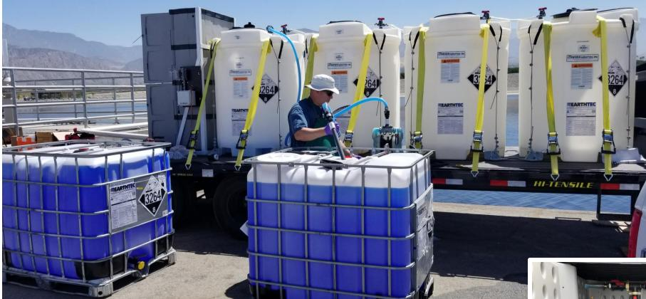
EarthTec liquid ionic copper, typically dosed with metering pumps. Mobile dosing trailer can be deployed for emergency or trial applications.
