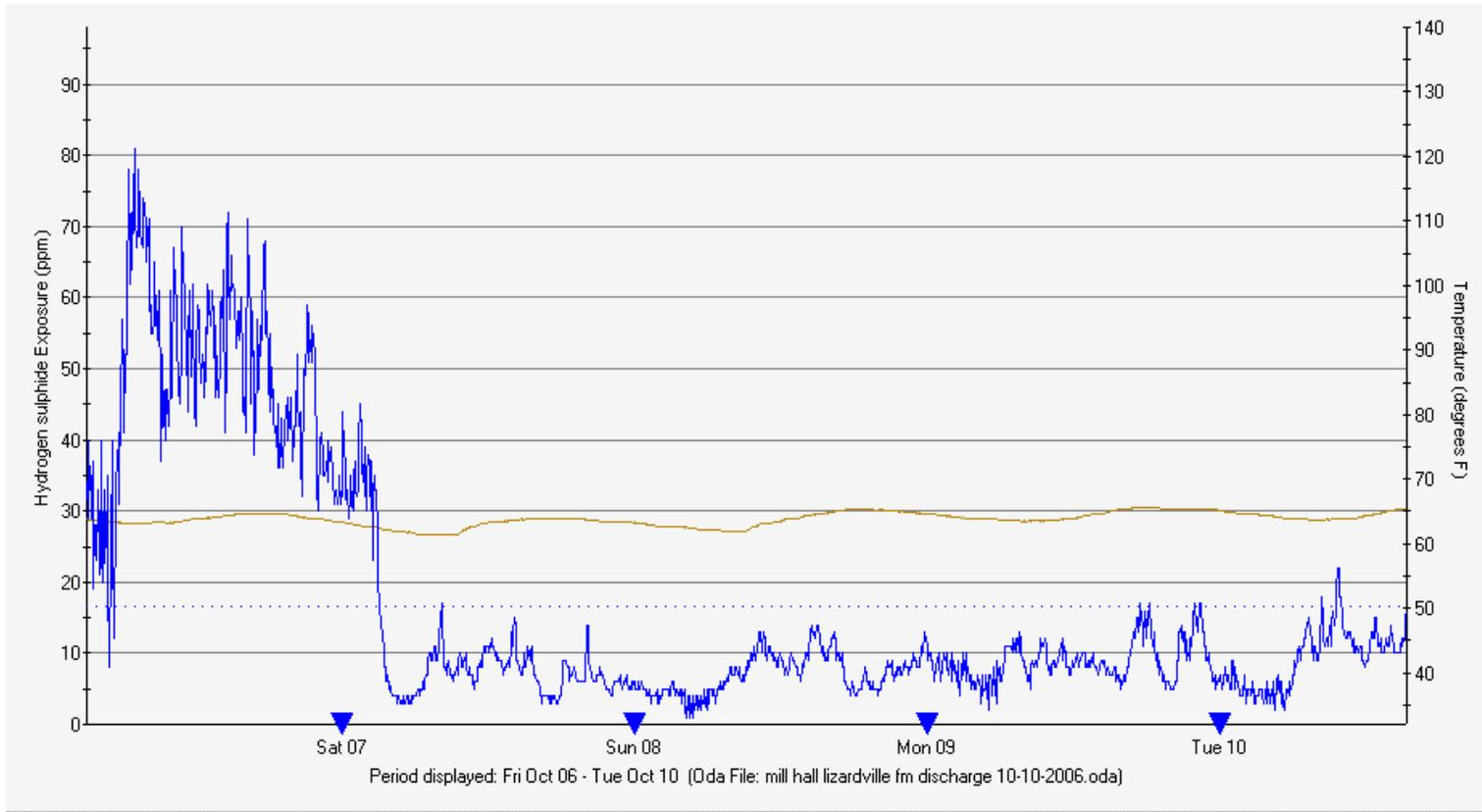
— INST : Min (1 ppm) Max (81 ppm)    ▼ Day Transition    ..... Average (16.6 ppm)    — Temperature
