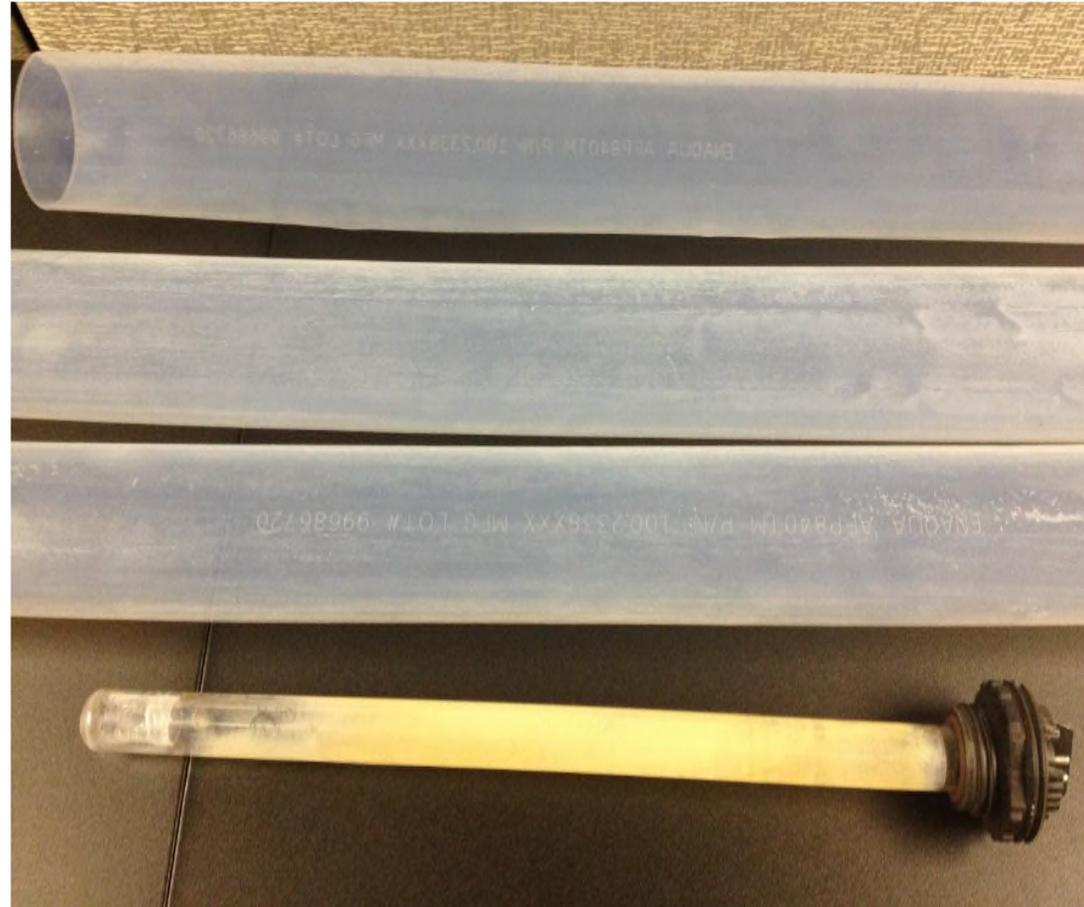
Figure 4 Comparison of New Tube (top) to Tubes and Quartz Sleeve after 73 Days
