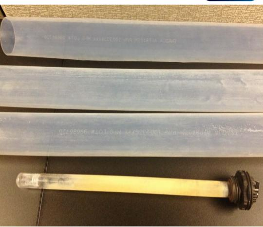
Figure 4 Comparison of New Tube (top) to Tubes and Quartz Sleeve after 73 Days
