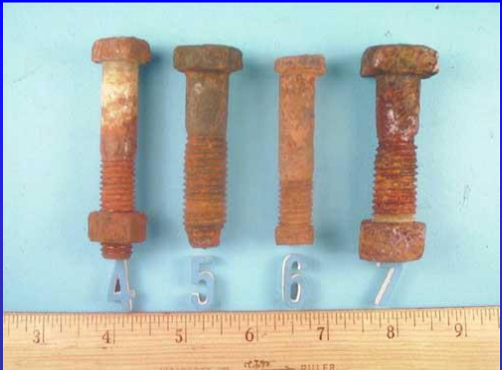
Bolt & Nut Corrosion
