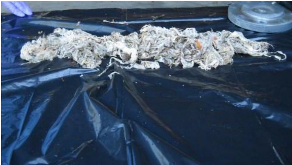
Pump clog debris
