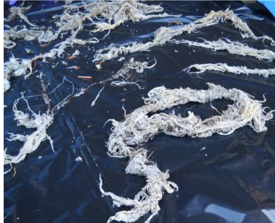
Decomposed debris clog
