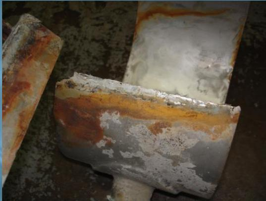
**Poor Passivation at the Welds and Too Many Welded Components**
