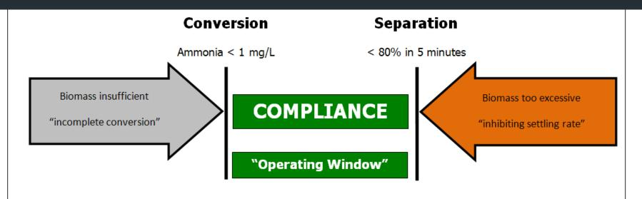
Establishing a wasting rate is simply a process of maintaining sufficient biomass
