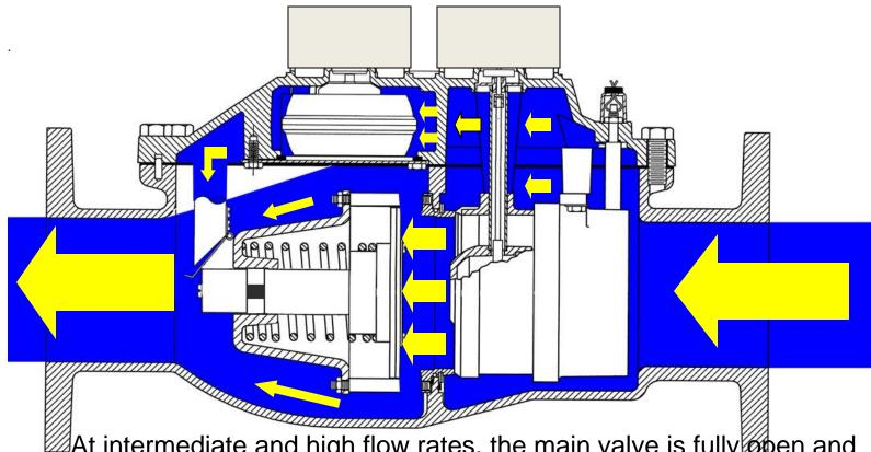
At intermediate and high flow rates, the main valve is fully been and the majority of the water flows through the turbine. Water continues to flow through the T-10 at a greatly reduced rate. This helps "flush" the the T-10 while simultaneously insuring that it does not "over-
