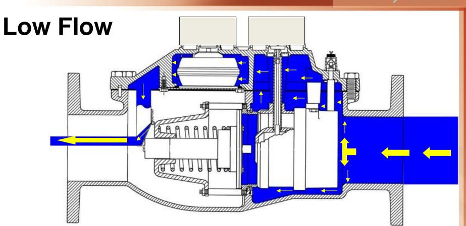
At low flow, the main valve prevents water from flowing through the Turbine element.
