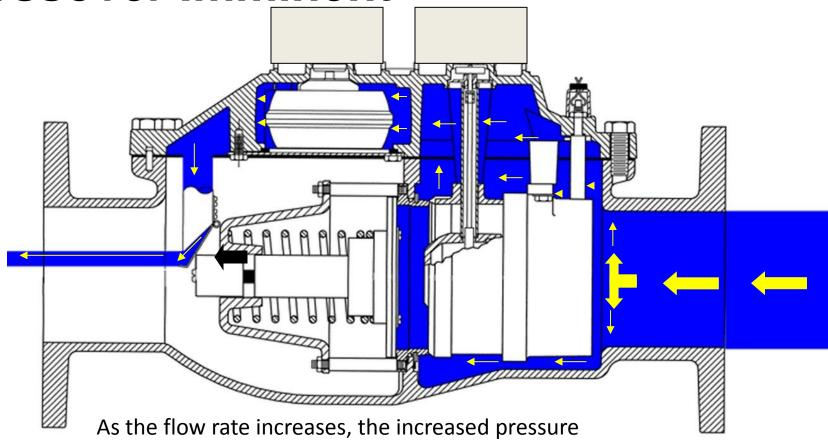
differential causes the valve piston to move rearward, closing the throttle tube door, reducing the flow through the T-10 chamber.
