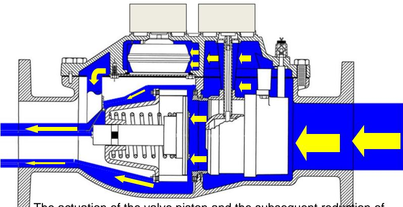
The actuation of the valve piston and the subsequent reduction of flow through the T-10 chamber "shunts" a large volume of water through the turbine measuring element forcing the main valve open. Both the turbine and the T-10 are operating.
