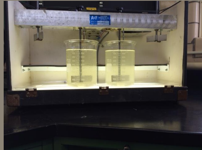
Jar Test at the Napoleon WWTP
