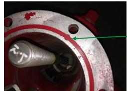
A hole is machined into the groove to allow a screwdriver to pry O-ring out without cutting the O-ring
