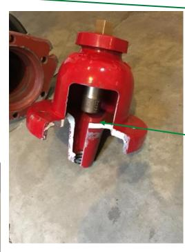
No need for a stop nut. This allows the bonnet to be spun off without taking any of the operating system apart.
