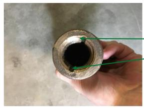
When lubricating the K81D, grease is forced down the length of the upper stem threads by grooves machined into the op nut.
