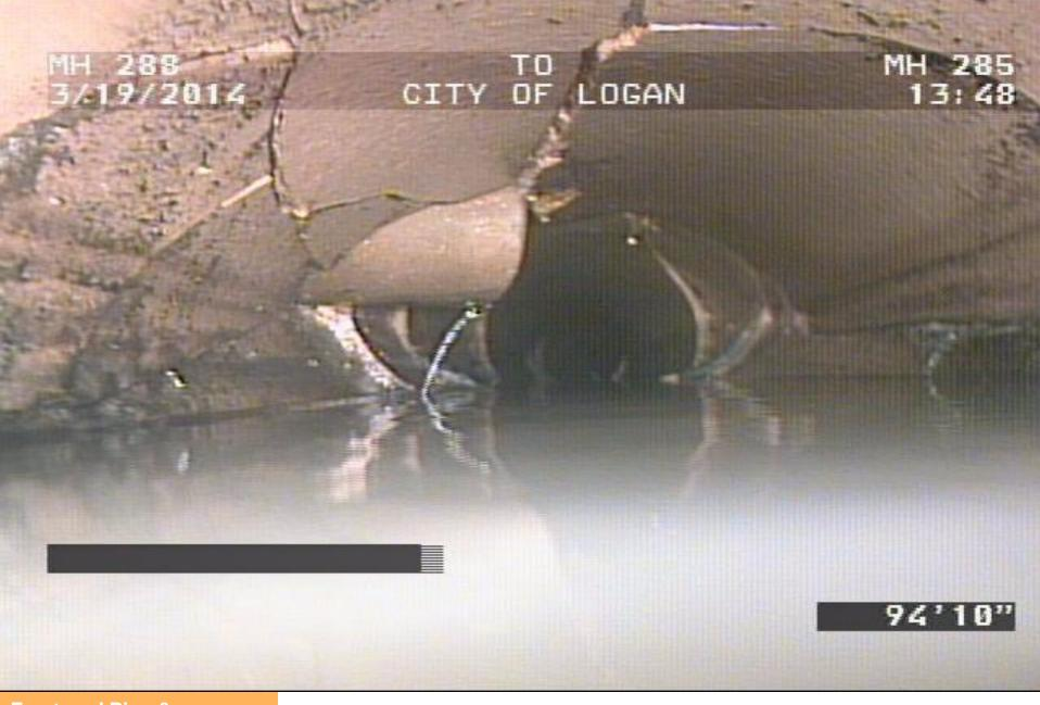
Fractured Pipe & Hammer Tap
