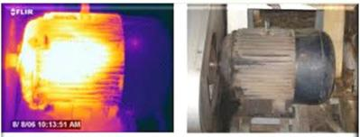
Above thermal and daylight images show a three phase motor which has overheated. Power quality analysis proved condition was caused by negative sequence harmonics.
