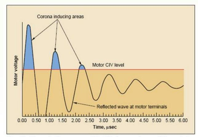
Figure 2 — The peak voltage can exceed the CIV value more than once during a single pulse. For example, any voltage over 1,600 V in a 480-V system will trigger a series of waves over the CIV level.
