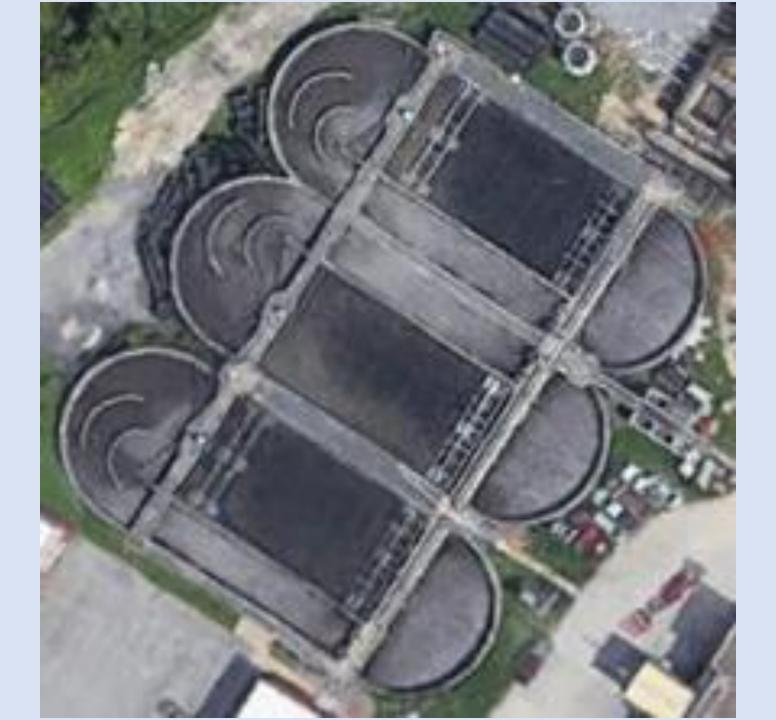
In 2017, the City upgrades their WWTP from a typical extended aeration system to modern Biological Nutrient Removal system.
