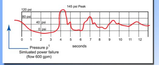
Simulated Power Failure with 2-1/2" 52 Series Surge Control Valve
