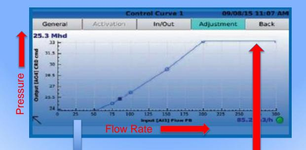
During times of low demand or at night, system pressure is reduced. • During times of high demand or during the day, system pressure is increased.
