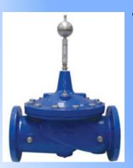
If air gets into the pilot system of a pressure reducing valve, the valve will lose the ability to regulate pressure, causing system pressure to increase, resulting in pipe breaks and/or increased leakage. An air release valve on the cover of the valve can help prevent this.
