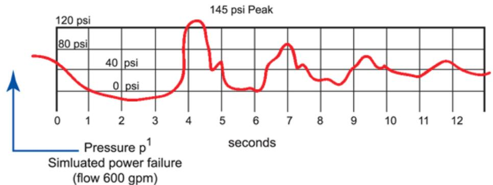
Simulated Power Failure with 2-1/2" 52 Series Surge Control Valve
