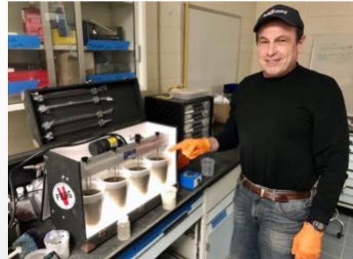
On the following page is an illustration of the results of jar testing done to determine how much  $MgOH_2$  slurry is needed to dissolve grease and break out to settle any debris that has been cemented into the grease blanket.
