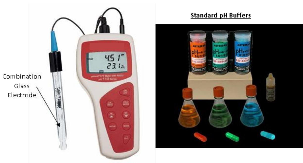
**Figure 3. Simple portable hand-held pH meter with combination glass electrode and standard pH buffers for calibration (red = pH 4.00, green = 7.00, blue = 10.00, all  $\pm 0.02$  units at 25°C)**
