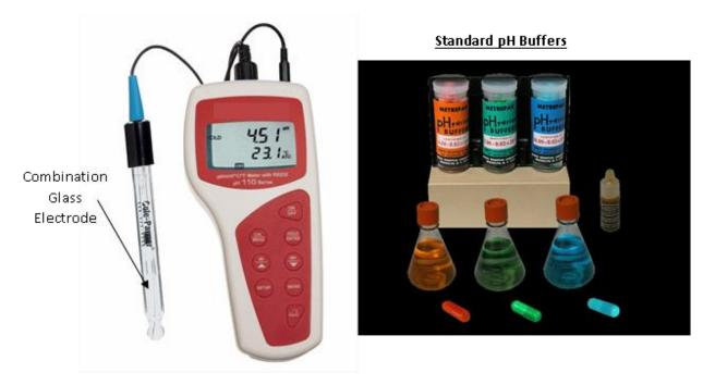
Figure 3. Simple portable hand-held pH meter with combination glass electrode and standard pH buffers for calibration (red = pH 4.00, green = 7.00, blue = 10.00, all ± 0.02 units at 25°C)
