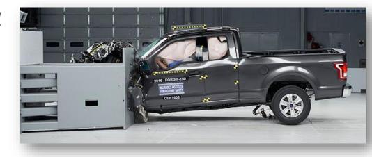
F150 truck weighing 4,000 lbs traveling at 55 mph hits a wall
