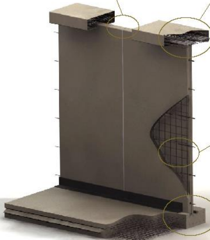
RECTANGULAR POST-TENSIONED TANK DETAILS
