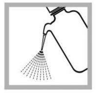
1. Rinse the probe with deionized water. Dry the probe with a lint-free cloth.
