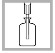
**4.** Remove the stopper. Put the probe in the bottle.
