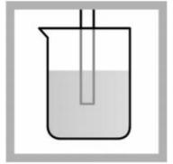
2. Laboratory test: Put the probe in a beaker that contains the solution. Do not let the probe touch the stir bar, bottom or sides of the container. Remove the air bubbles from under the probe tip. Stir the sample at a slow to moderate rate. Field test: Put the probe in the sample. Move the probe up and down to remove bubbles from the electrode. Make sure to put the
