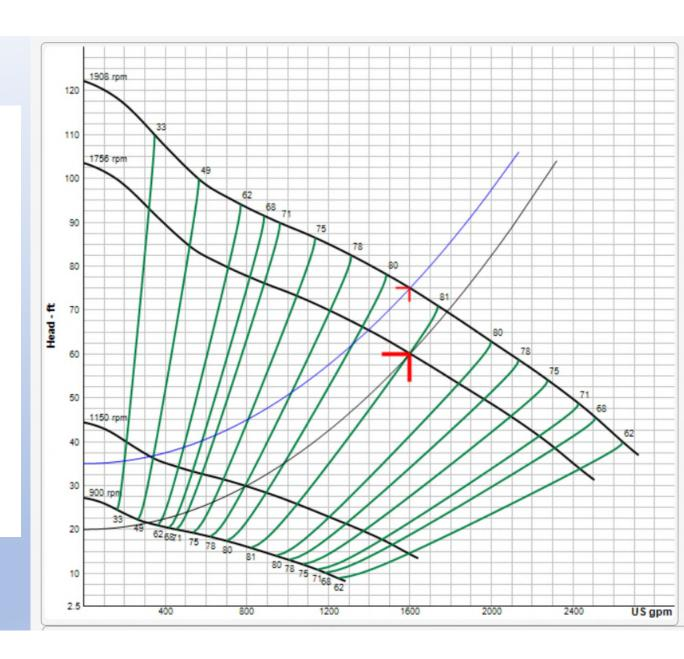
In this graph, there are two system curves. The design point is the same, but the \_\_\_\_ is different.
